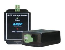
The **4-20mAmp** signal converter is used to integrate the sensorProbe or securityProbe with a **4-20mAmp** transmitter. **4-20mAmp** technology is used to communicate analog signals over long distances where electrical interference is a problem. This solution is often used in the process control industry to collect the analog values from a wide array of remote sensors.
