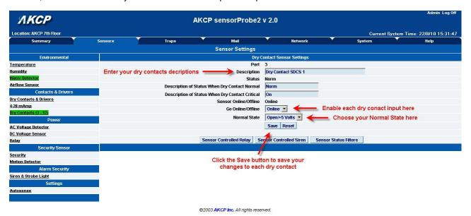
Now enter your all of your dry contacts descriptions, descriptions of status (if you don't see this, note the reason below), enable all the dry contacts, the normal state then save your configurations. Note: the 5DCS dry contacts can only be setup as inputs and cannot be setup as outputs. Maximum input is 5VDC.
