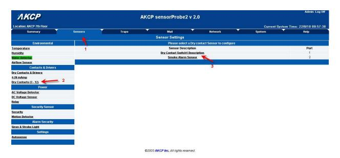
Click on the Sensors page, then click on the Dry Contacts (3 - 12) in the "Contacts & Drivers" column, then click on the dry contact switch Description on port 1 as shown above.
